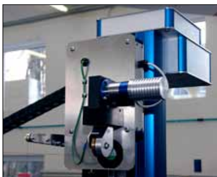
■ The wire tensioning system with motor or sensor unit ensures constant wire tension irrelevant of the portal distance and angular position. The fans for active wire cooling in the external range can also be seen clearly.
