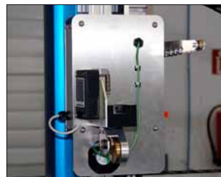
■ The wire tensioning system with motor or sensor unit ensures constant wire tension irrelevant of the portal distance and angular position. The fans for active wire cooling in the external range can also be seen clearly.
