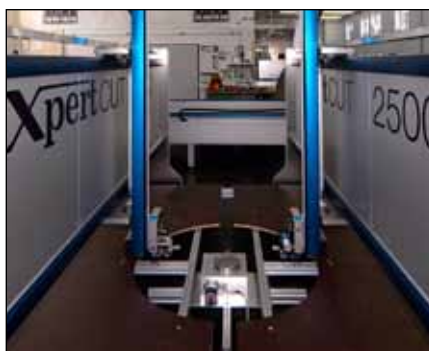
■ The software controlled portal adjustment allows an extremely fast adjustment of the portal distance to the work piece dimension.
