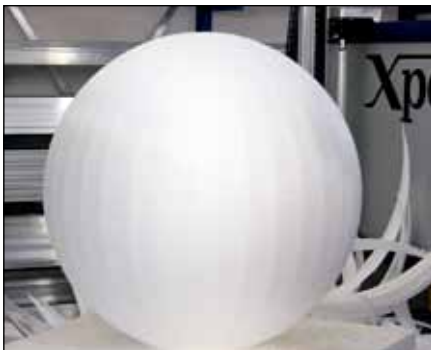
■ Test cut of a spherical shape on the Xpert CUT 2500.
