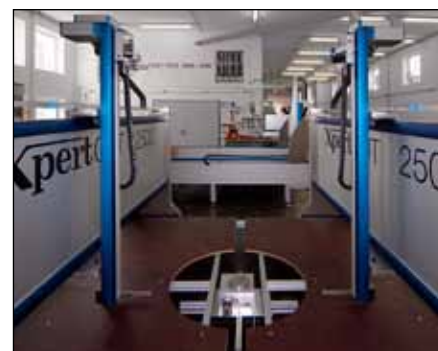
■ The software controlled portal adjustment allows an extremely fast adjustment of the portal distance to the work piece dimension.
