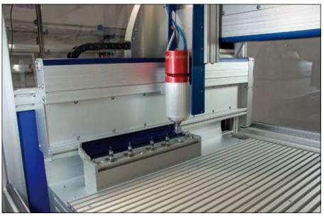
Milling spindle and tool station on the Xpert 3D
