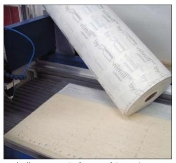
vilmill increases the fixation of the work piece.
