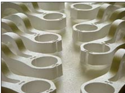
■ Cast aluminium molds made of polystyrene
