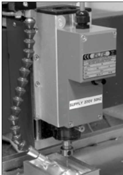
■ ELTE electric spindle with incorporated inverter.
