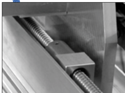
■ ball-bearing spindle in Precise 1000 U
