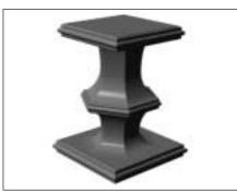
■ Figure : Only three simple cutting contours are needed to produce this column.
