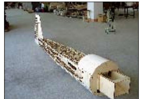
■ The YAK 54 is made entirely of wood.
