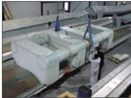
■ Base for the rotor blade created using hot-wire cutting technology.
