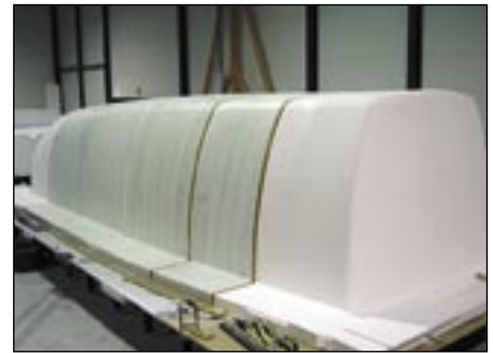
■ Prototype model of the casing of a wind turbine.
