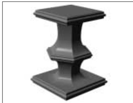
■ Figure 1: Only three simple cutting contours are needed to produce this column.
