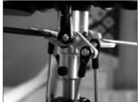
■ Mr. Licha uses his Basic 540 milling unit to mill all sorts of things incl. mixing levers.
